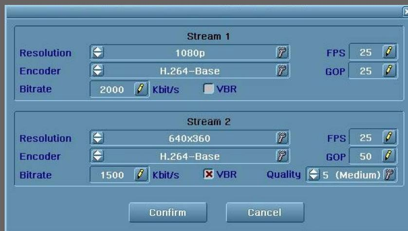
The screenshot shows a configuration window with two sections for Stream 1 and Stream 2. Each section has fields for Resolution, Encoder, Bitrate, FPS, and GOP. Stream 1 is configured with 1080p resolution, H.264-Base encoder, 2000 Kbit/s bitrate, and FPS of 25. Stream 2 is configured with 640x360 resolution, H.264-Base encoder, 1500 Kbit/s bitrate, FPS of 25, and GOP of 50. A Quality dropdown is set to 5 (Medium). There are Confirm and Cancel buttons at the bottom.
